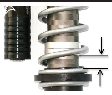
Crossover ring placement value should match the distance from the top of the spring coupler to the bottom of the crossover ring. Example .912 inches
