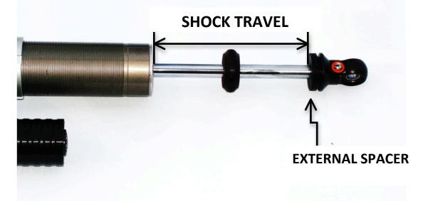
SOME SHOCKS USE EXTERNAL SPACERS BELOW THE BUMP STOP TO LIMIT TRAVEL. DO NOT INCLUDE THE SPACER LENGTH AS PART OF THE TRAVEL.
